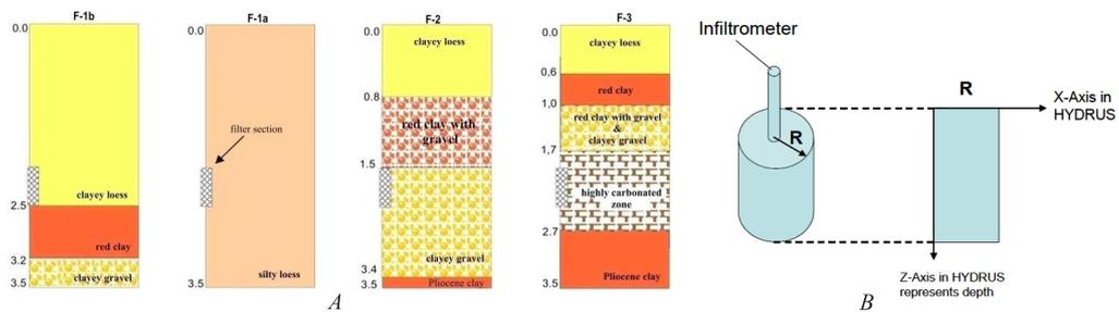
Fig. 4. A) Conceptual models used in the axisymmetric flow calculations. Vertical dimensions (in metres) refer to model coordinates. B) Axisymmetrical flow model with radially finite, 3D geometry, applied to each of the conceptual models
