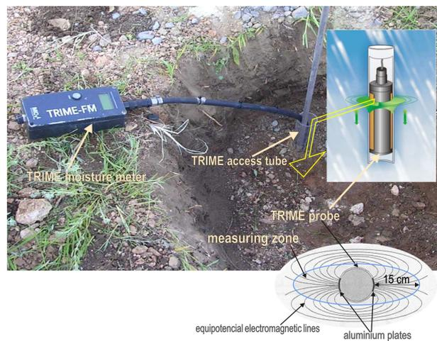
Fig. 3. Time-domain reflectometry apparatus (TRIME T3-44) for volumetric soil moisture measurements
