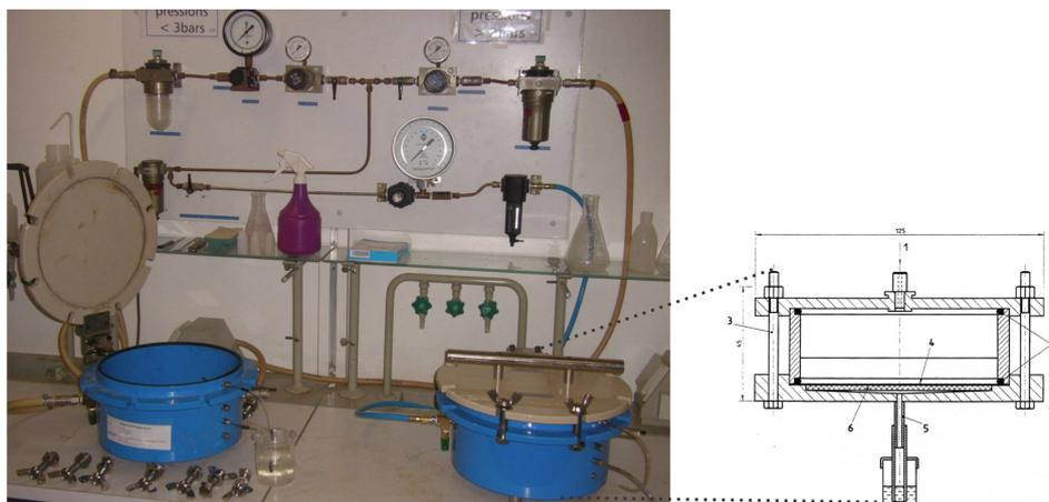
Fig. 1b. Pressure membrane cell for soil water suction determination  $> pF\ 2$  [20]: 1 – air from compressor; 2 – O-rings; 3 – bolts; 4 – visking membrane; 5 – outflow pipe; 6 – sintered bronze plate
