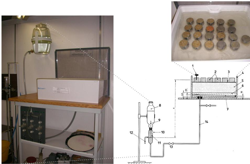
Fig. 1a. Sand suction table for soil water suction determination up to  $pF\ 2$  [21]: 1 – tensiometer; 2 – soil core sample; 3 – nylon voile; 4 – ceramic sink; 5 – fine sand; 6 – coarse sand; 7 – drain system; 8 – reservoir; 9 – thin nylon tube; 10 – air inlet; 11 – levelling bottle; 12 – overflow; 13 – tap; 14 – flexible nylon tubing
