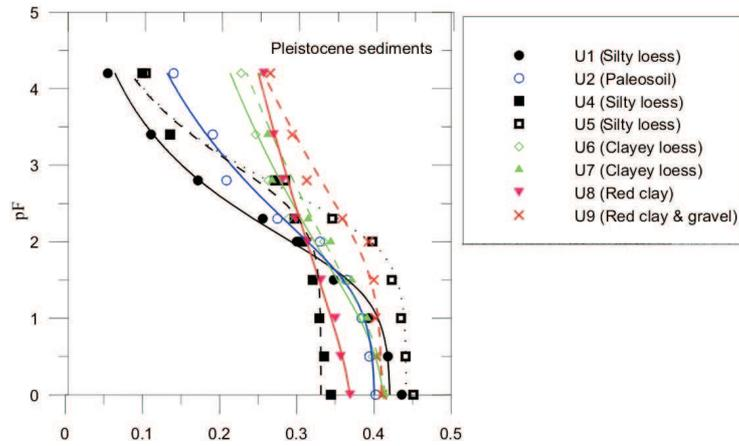
Fig. 2. Measured (symbols) and fitted van Genuchten moisture retention curves
